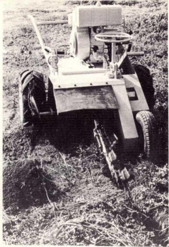
The Wenco hydraulically driven pedestrian trencher.
